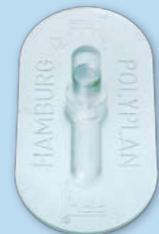
Adhesion packer oval (1131 A) made of transparent polycarbonate, size 50 x 100 mm, outside thread M 10 x 1.0 weight circa 15 g
