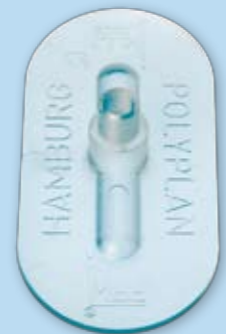
Adhesion packer oval (1131) made of transparent polycarbonate, size 50 x 100 mm, inside thread M 8 x 1.0 weight circa 15 g
