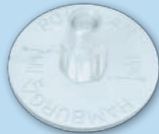
Adhesion packer round (1138) made of transparent polycarbonate, 48 mm Ø, inside thread M 8 x 1.0 weight circa 7 g
