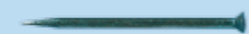
Steel pins (1137) with smoothed tips and countersunk heads for centering the adhesion packers, they prevent slipping on vertical surfaces. 2 mm Ø, 40 mm long, 100 per bag
