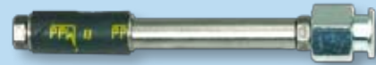
(1013 LF) 13 mm Ø, overall length 115 mm, thread M 6 with flat-head nipple (1120 C)
